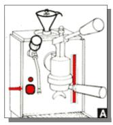
A Unscrew the cap of the boiler (1) and fill with fresh water up to the upper level of the water-level indicator (2). Screw on the cap of the boiler (1). Turn off the steam tap (3), by turning it to the right. Plug into the mains. Press the switch (4) and its light, and the indicator light of the automatic water-heater (5) will go on.
