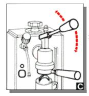
Preheat the filter-holder (6), by attaching it to the piston-head (9) moving the handle of the filter-holder (8) to the right and releasing a little hot water by raising the piston-lever (7).
